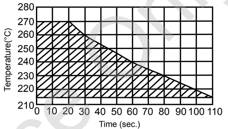
(6) Recommendable Temperature Profile for Soldering
