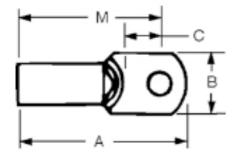
These non-insulated ring terminals are made of electrolytic copper for high conductivity. They can be installed with crimping tools having a single indentor or double indentor (recommended for solid
