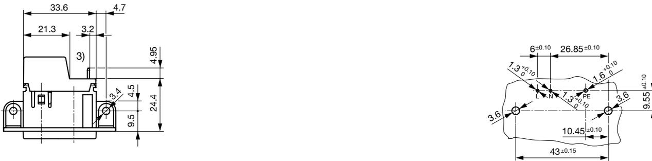
3) PE additionally as quick-connect terminal 4.8 x 0.8 mm
