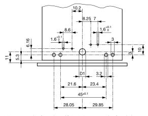
Fixation on PCB or housing from below
