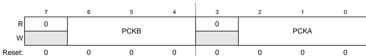
Figure 26-5. PWM Prescale Clock Select Register (PWMPRCLK)
