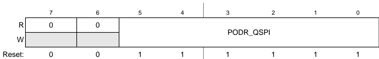
Figure 13-5. Port QSPI Output Data Register (PODR_QSPI)
