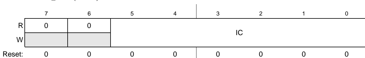
Figure 32-3. I 2 C Frequency Divider Register (I2FDR)
