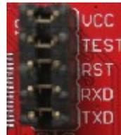
**Figure 37. eZ430 Debug Connector on MSP-EXP430G2 LaunchPad**
