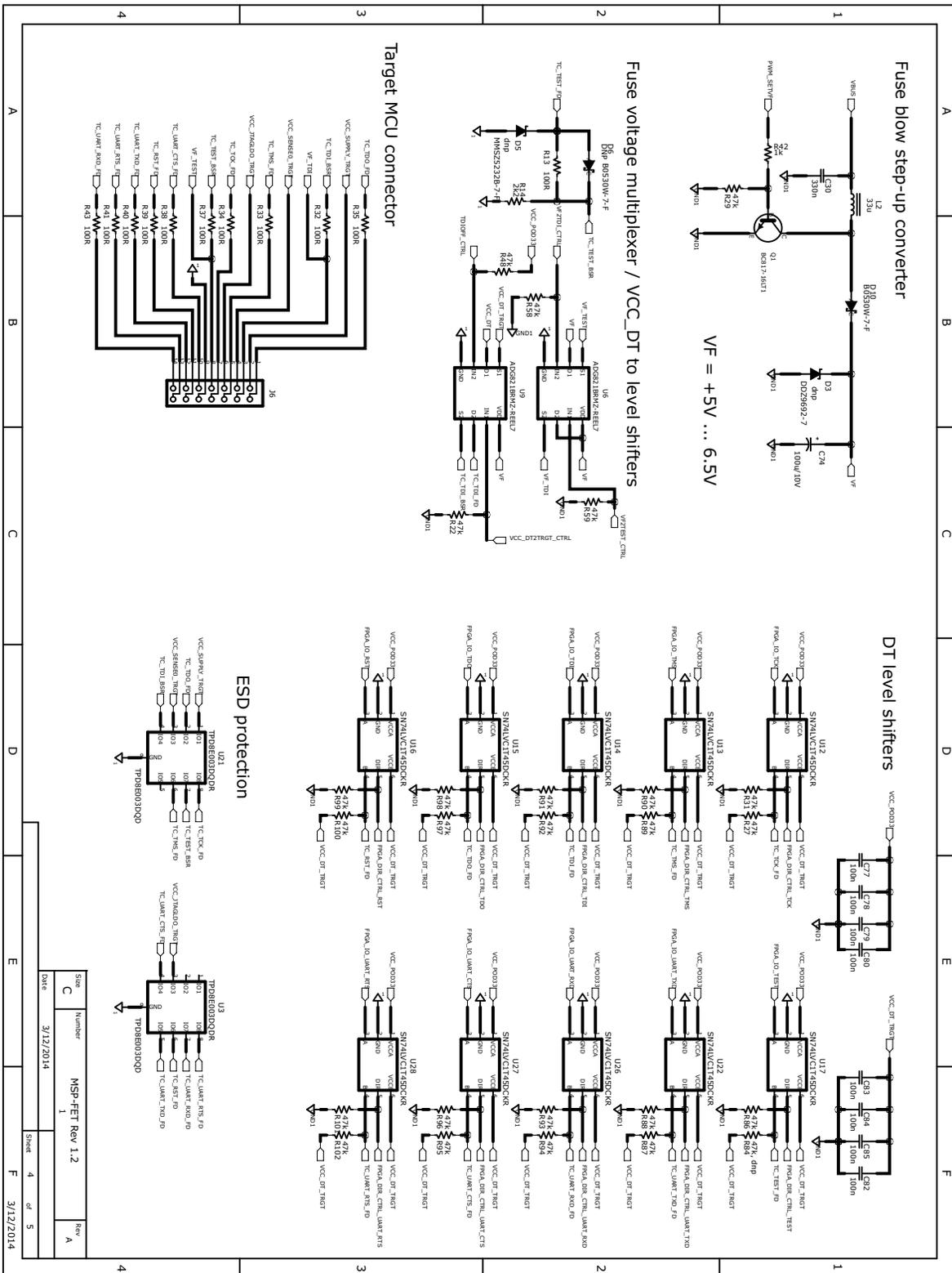
Figure 16. MSP-FET USB Debugger, Schematic (4 of 5)
