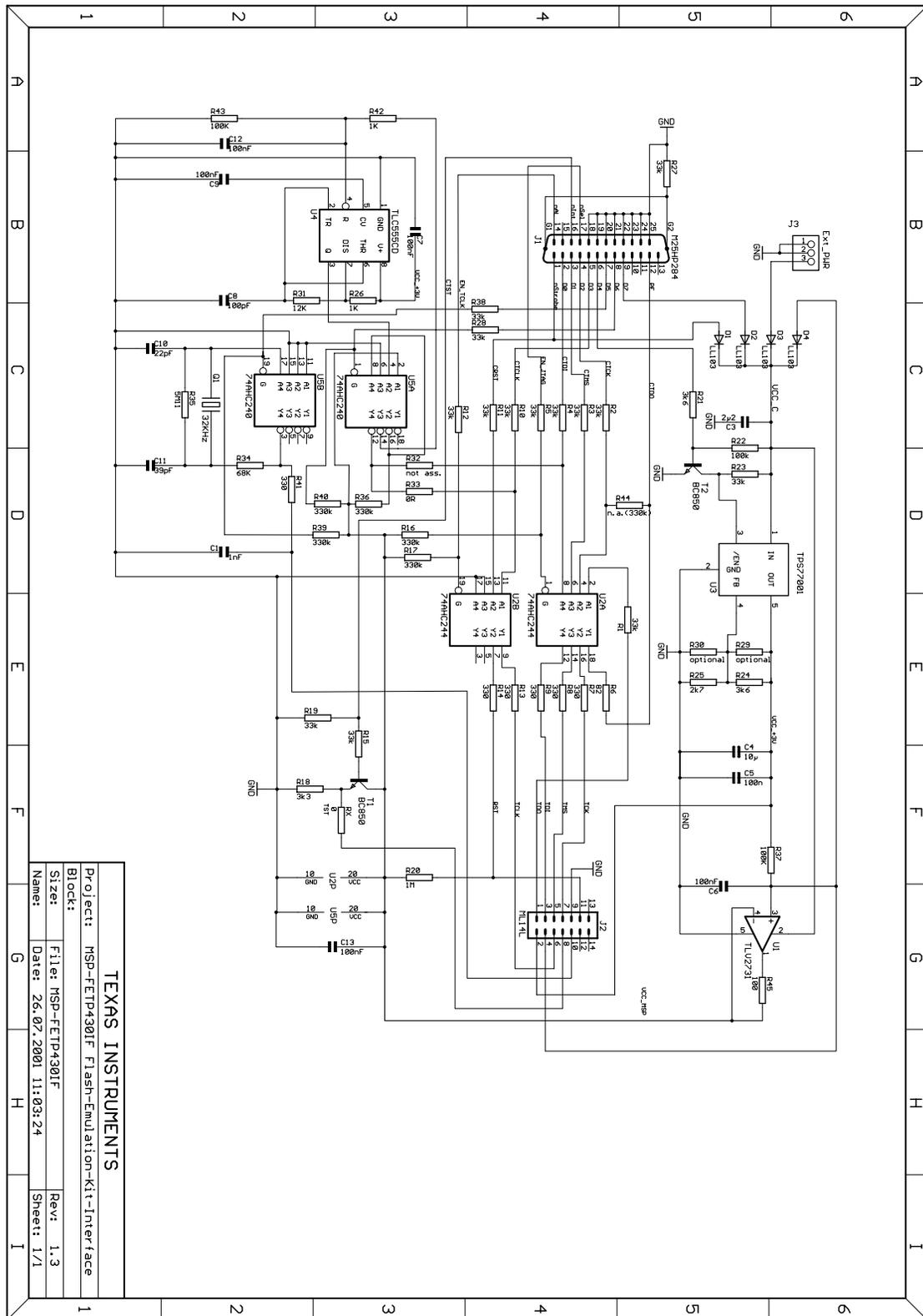
Figure 41. MSP-FET430PIF FET Interface Module, Schematic
