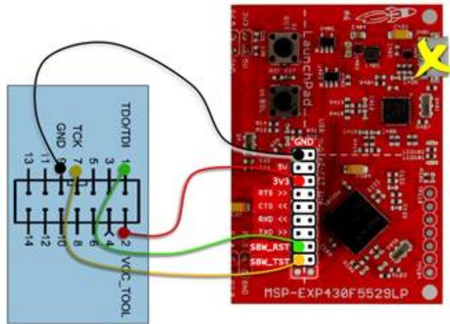
Figure 31. MSP-FET to LaunchPad Pin Assignments
