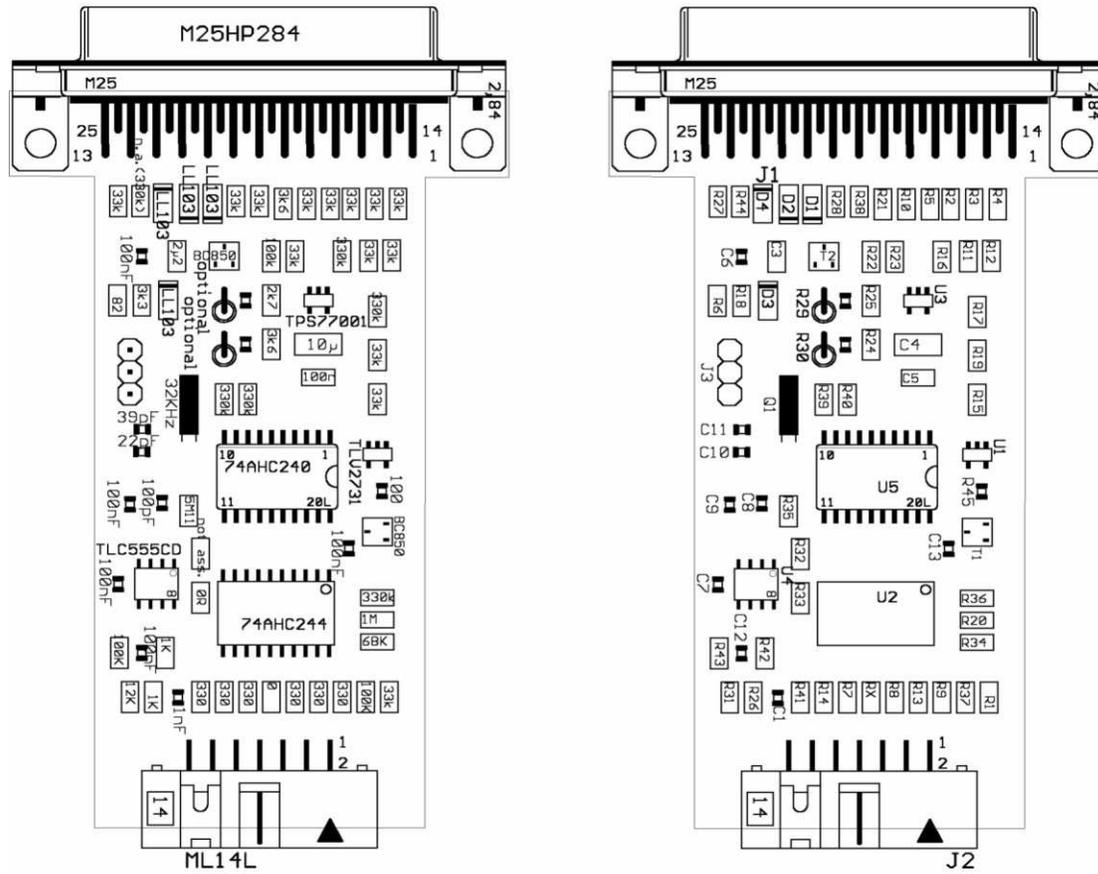
Figure 42. MSP-FET430PIF FET Interface Module, PCB
