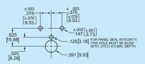
Panel Mounting Detail: Tolerance for Mtg. ±.005 [.13] Panel Thickness: .125-.156 [3.18-3.96]
