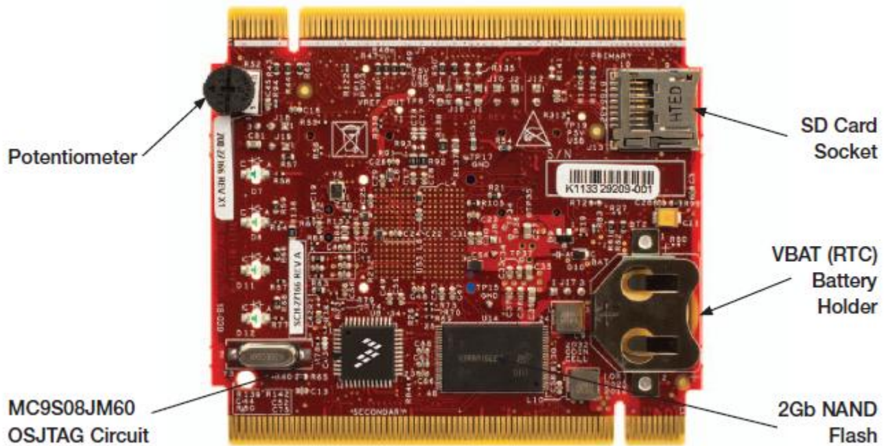
Figure 3. Callouts on back side of the TWR-K70F120M
