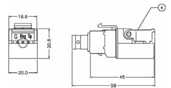
Connections are made by simply lifting the plastic tab (4) and exposing the insulation displacement connector. Individual Cat5 conductors should be placed in the ring and tip slots of this connector. After lying the conductors in the slots, simply snap the plastic tab (4) back into place. This IDC connector is designed to pierce the insulation, **DO NOT** remove insulation from the end of the conductors.
