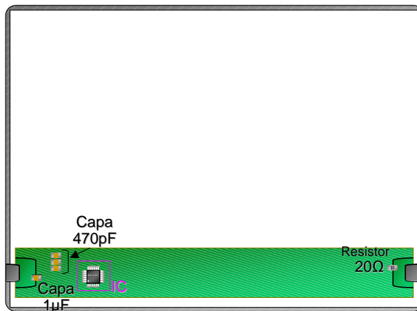
Figure 41. Layout example for ESD protection
