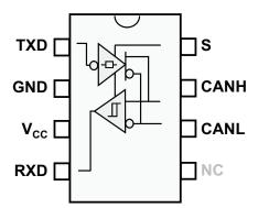
Figure 3. SN65HVD255 Basic Block Diagram & Pin Out
