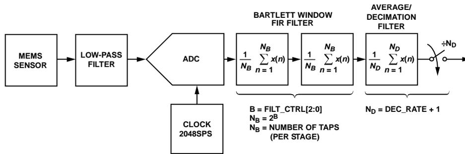
Figure 30. Sensor Sampling and Frequency Response Block Diagram
