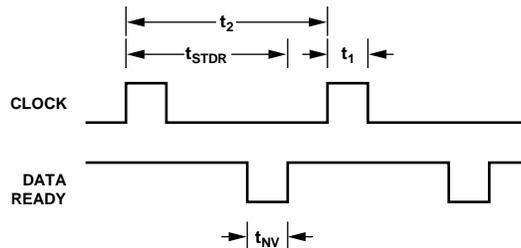
Figure 4. Input Clock Timing Diagram, MSC\_CTRL[0] = 1
