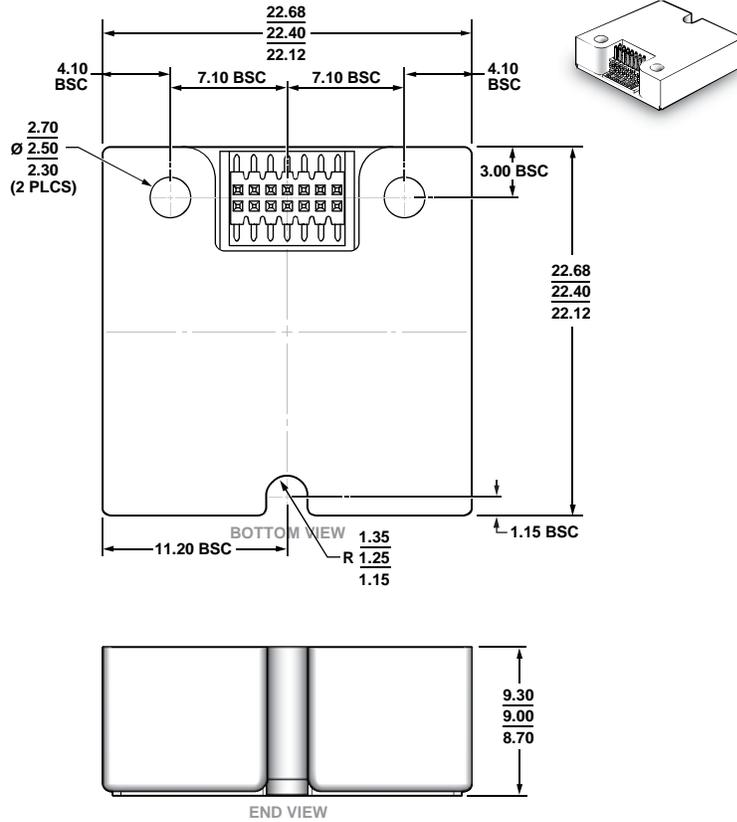
Figure 37. 14-Lead Module with Connector Interface [MODULE] (ML-14-5)
