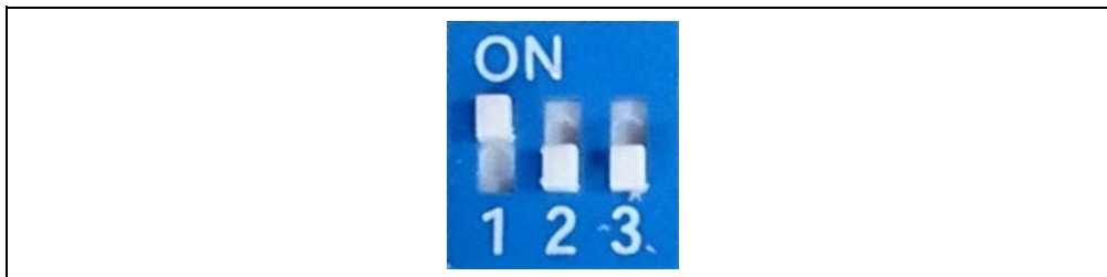
FIGURE 3-29: SWITCH SW9 IN TEST MODE
