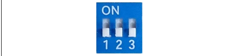
FIGURE 3-1: SW9 IN FLASH APPLICATION MODE
