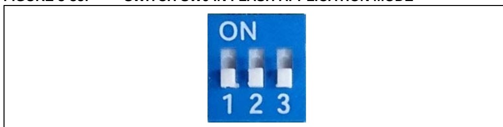
FIGURE 3-35: SWITCH SW9 IN FLASH APPLICATION MODE
