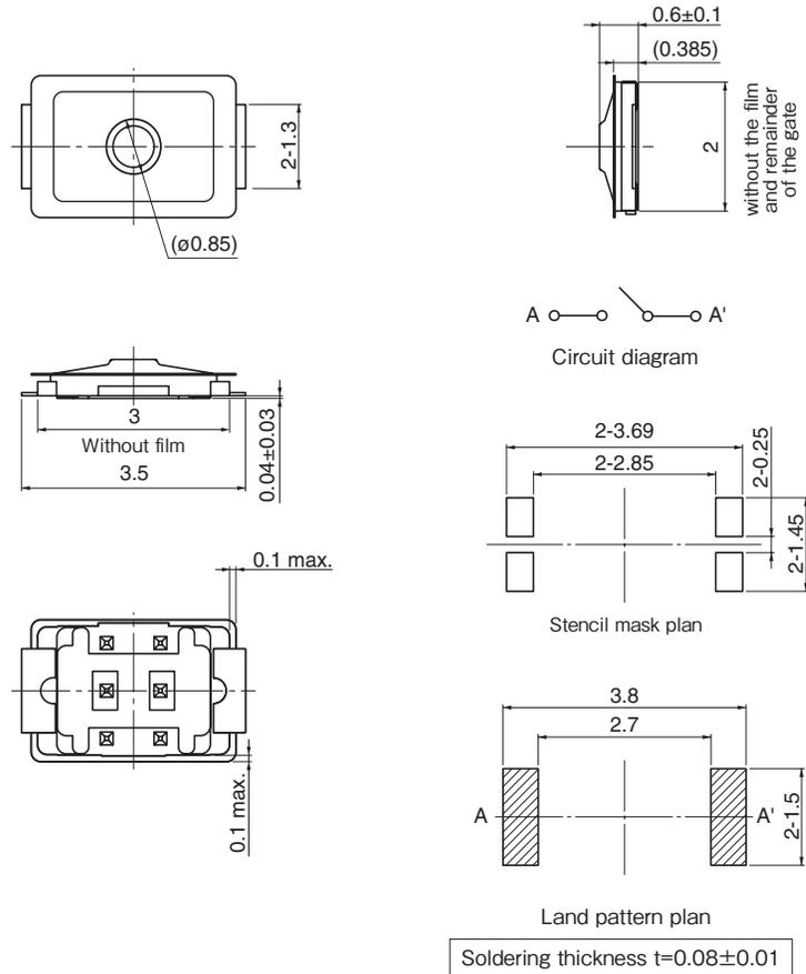
\*Soldering failure may occur depending on applied solder amount, so, please consider to use our recommended stencil and land pattern desing.
