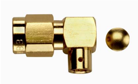
Model 72959 SMA PLUG R/A CRIMP, RG141, 174, 188, 316
