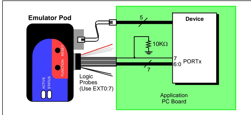
For this trace configuration, seven (7) lines of data and one (1) line for clock are transmitted. PORTx must be a port with eight pins that has all eight pins available for trace. The port does not have to be one physical port but can be made up of pins from more than one port. The port pins must not be multiplexed with the currently-used PGC and PGD pins.
