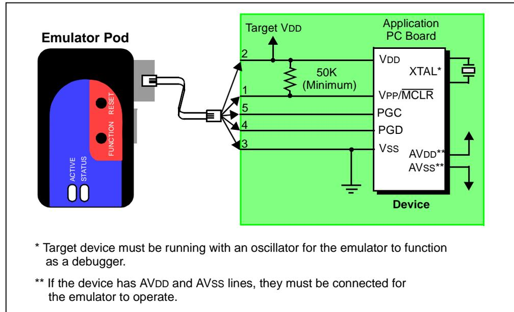
In the following descriptions, only three lines are active and relevant to core emulator operation: pins 1 (VPP/MCLR), 5 (PGC) and 4 (PGD). Pins 2 (VDD) and 3 (VSS) are shown on the above diagram for completeness, but are only sensed, not provided or controlled, by the emulator.
