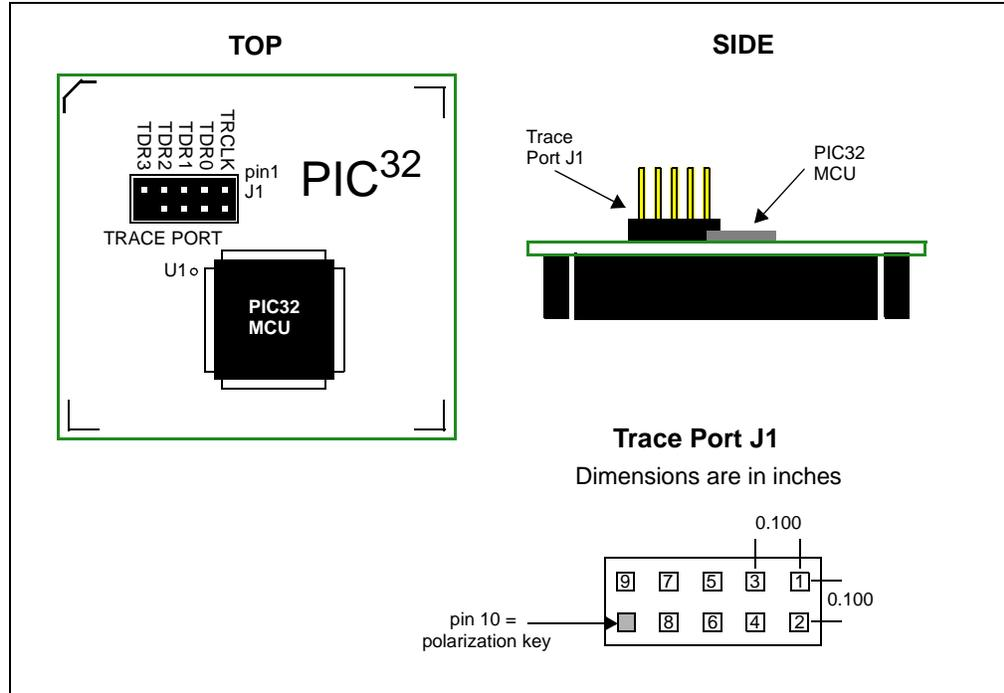
**FIGURE 15-2: PIC32 PIM PIN CONNECTION DIAGRAM**
