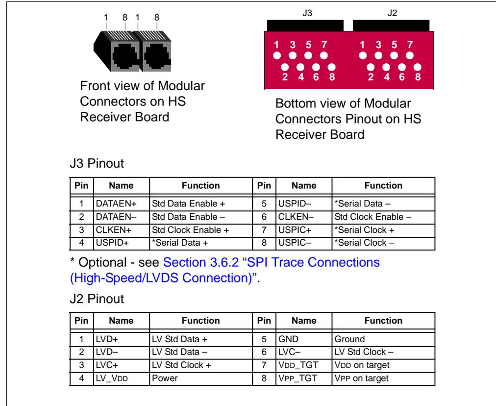
**FIGURE 13-3: 8-PIN HEADER PINOUT OF HIGH-SPEED RECEIVER BOARD**
