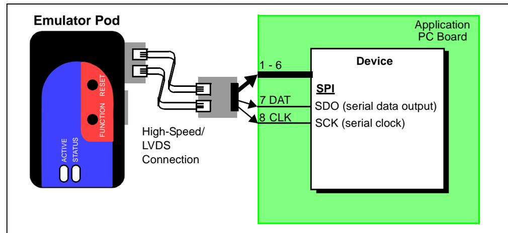
The DAT and CLK lines are intended for use with devices that do not have built-in debug logic that allows tracing (Native trace) to use the PGD/PGC/EMUC/EMUD pins. The DAT line connects to either the target device SPI port SDO1 or SDO2. The CLK line connects to SCK1 or SCK2.
