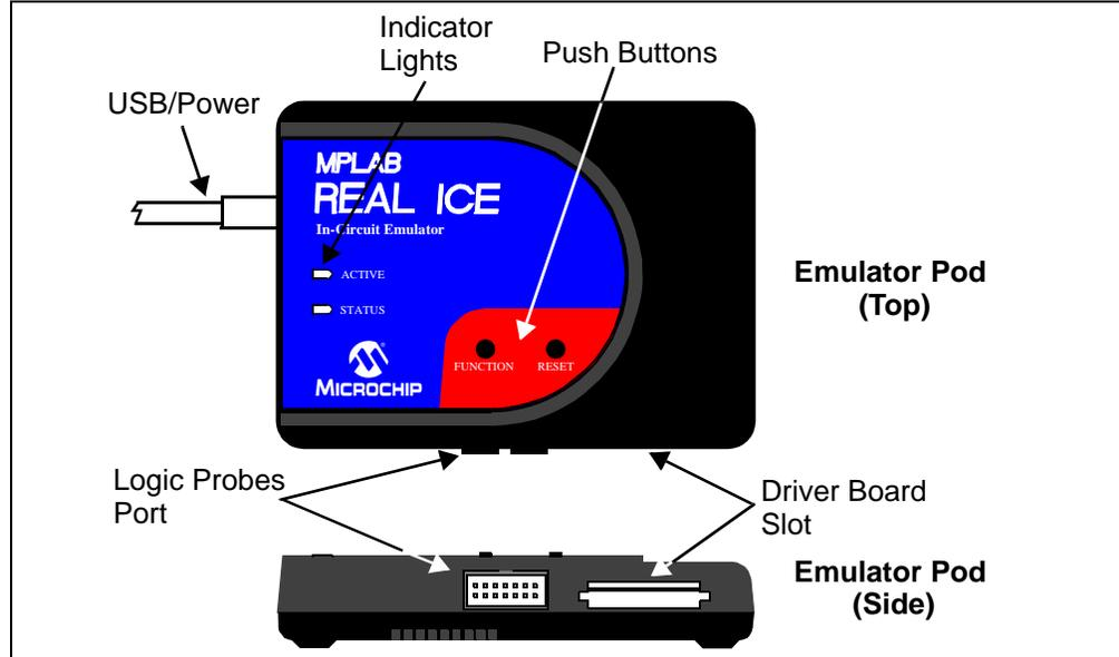
The emulator communicates with the PC and is powered through the USB cable.
