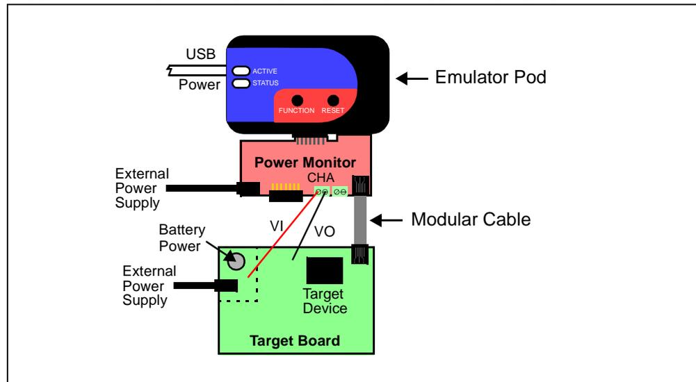
**FIGURE 22: CHA INTERNAL CONNECTIONS**
