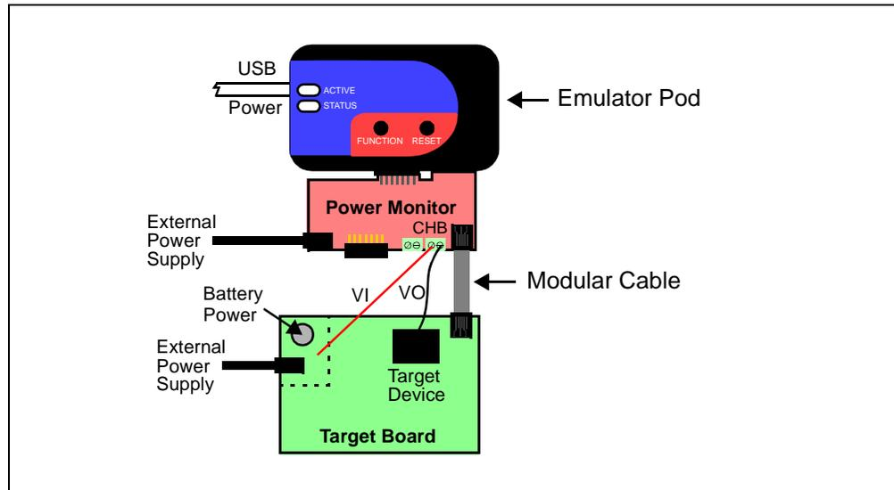
FIGURE 24: CHB INTERNAL CONNECTIONS
