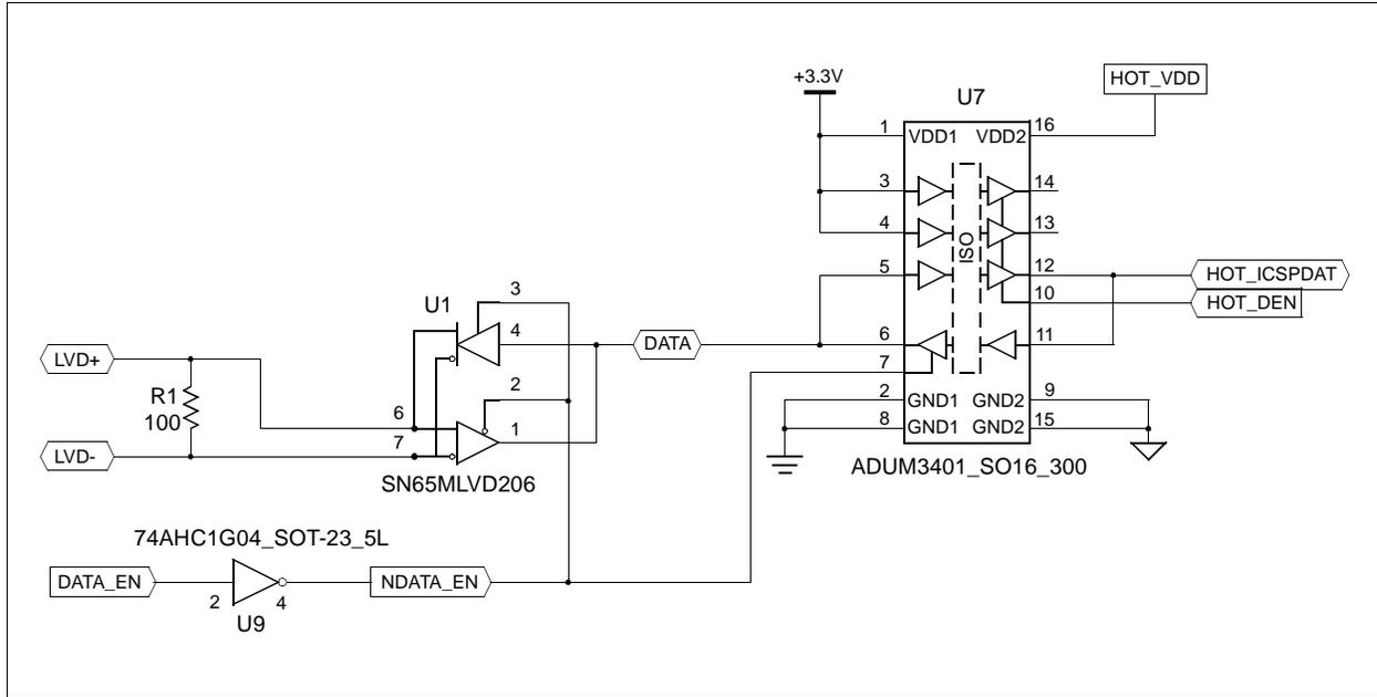
FIGURE 17-3: ISOLATOR UNIT SCHEMATIC – ICSPCLK
