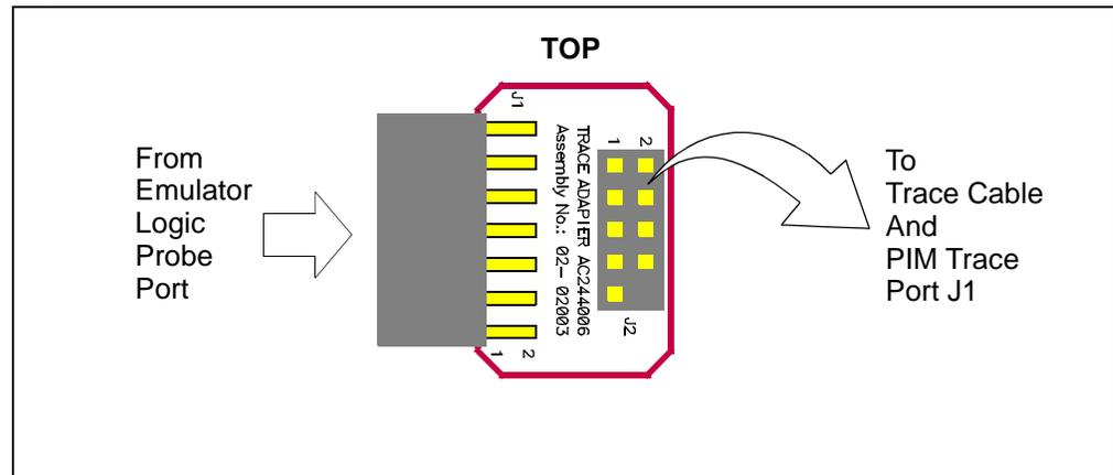
**FIGURE 16-2: ADAPTER BOARD PIN CONNECTION DIAGRAM**
