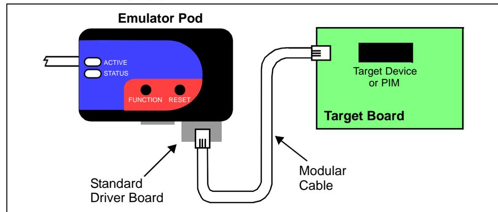
FIGURE 3-3: STANDARD CONNECTION – ICE DEVICE
