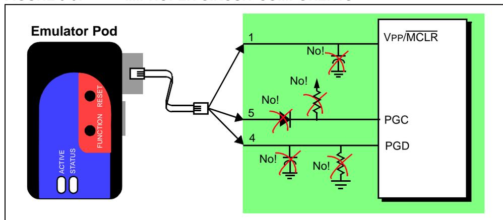
**VPP/MCLR pin:** do not use capacitors on  $\overline{\text{MCLR}}$  – they will prevent fast transitions of VPP. A simple pull-up resistor is generally sufficient.
