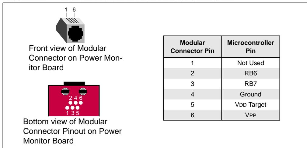
**FIGURE 22: MODULAR CONNECTOR PINOUT OF TARGET BOARD**
