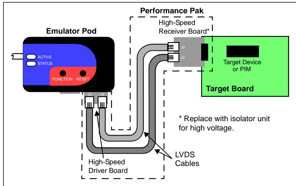
**FIGURE 3-5: HIGH-SPEED/LVDS CONNECTION – ICE DEVICE**
