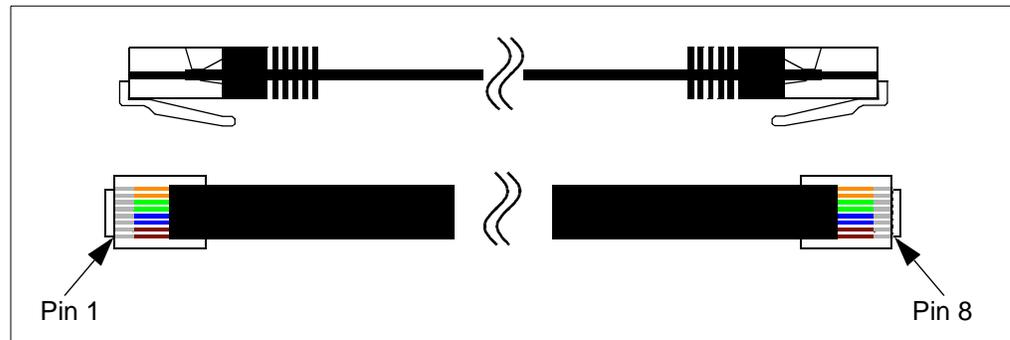
The target board should have the following 8-pin connection pinout to plug into the receiver board.
