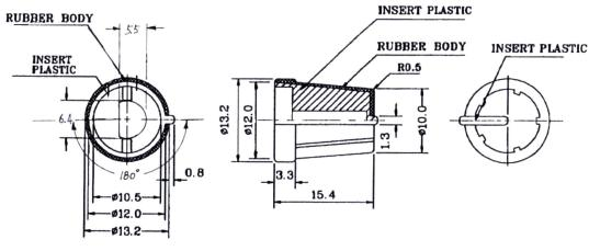
Dimensions : Millimetres Tolerance ±0.2mm
