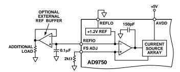
Figure 18. Internal Reference Configuration
