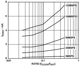
Figure 27. I<sub>DVDD</sub> vs. Ratio @ DVDD = 3 V
