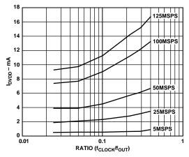
Figure 26.  $I_{DVDD}$  vs. Ratio @ DVDD = 5 V
