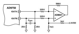
Figure 30. Single-Supply DC Differential Coupled Circuit
