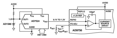
Figure 20. Single-Supply Gain Control Circuit
