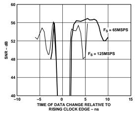
Figure 24. SNR vs. Clock Placement 2  $f_{OUT}$  = 10 MHz
