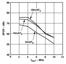
Figure 8. SFDR vs. f<sub>OUT</sub> and I<sub>OUTFS</sub> @ 25 MSPS and 0 dBFS
