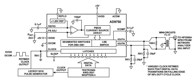
Figure 2. Basic AC Characterization Test Set-Up
