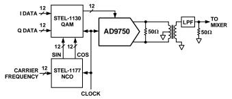
Figure 37. Digital QAM Architecture
