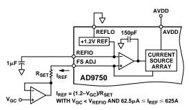
Figure 21. Dual-Supply Gain Control Circuit
