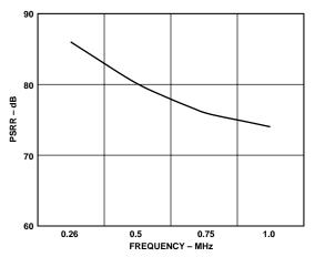
Figure 33. Power Supply Rejection Ratio of AD9750
