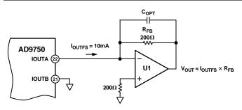
Figure 32. Unipolar Buffered Voltage Output
