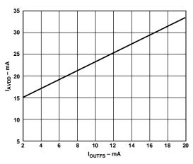
Figure 25. I<sub>AVDD</sub> vs. I<sub>OUTFS</sub>
