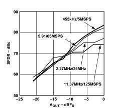
Figure 9. Single-Tone SFDR vs.  $A_{OUT}$ @  $f_{OUT} = f_{CLOCK}/11$
