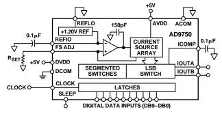
The AD9750 is a current-output DAC with a nominal full-scale output current of 20 mA and > 100 k $\Omega$  output impedance.
