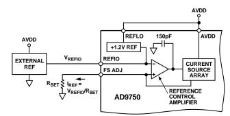
Figure 19. External Reference Configuration
