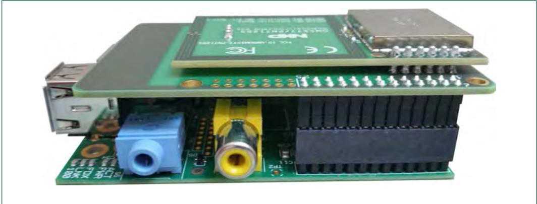
Fig 3. OM5577/PN7120S and Raspberry Pi B model stacked together
