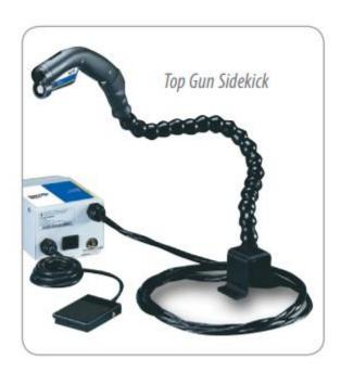
The Top Gun with Sidekick offers hands-free operation and flexible positioning during assembly and manufacturing processes. A foot pedal controls both ionization and airflow, which reduces compressed air costs and extends the life of the ionizer. The flexible gun mount allows the operator to focus the ionized airflow where it is needed. The stand includes a steel bracket for easy bench-top mounting.
