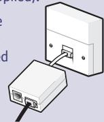
You'll need a microfilter for every phone socket where you've got equipment plugged in – up to a maximum of four per line – including alarm systems and digital TV boxes.
