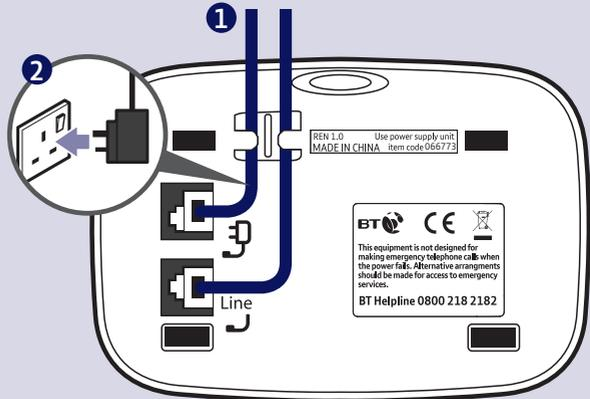
The phone line cord is pre-installed but **don't** plug the other end into the wall socket yet.
