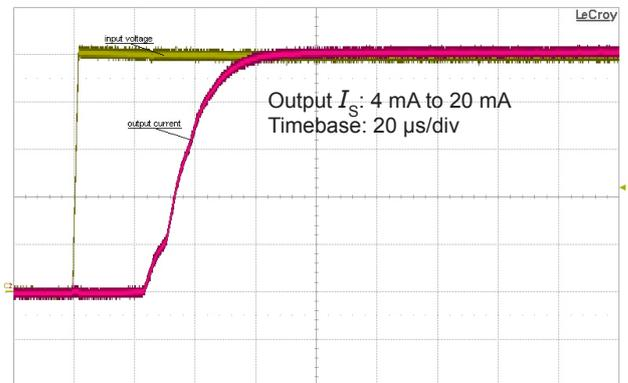
Figure 6: Typical step response (0 to  $V_{PN}$ )
