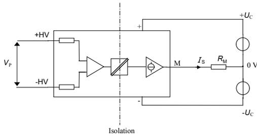
Figure 12: Standard characterization schematics for current output transducers ( $R_M = 50 \Omega$  unless otherwise noted)
