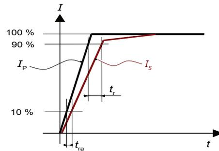
Figure 13: Response time  $t_r$  and reaction time  $t_{ra}$
