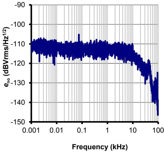
Figure 10: Typical noise voltage spectral density  $e_{no}$  with  $R_M = 50 \Omega$
