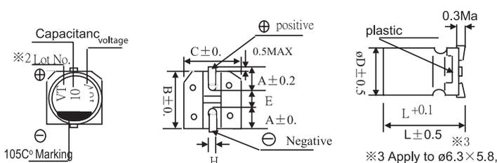
\*1. Voltage mark for 6.3V is [6V] Capacitance mark for 10 is  $10\mu\text{F}$ .
