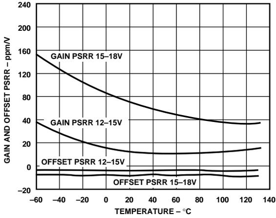
Figure 1. Gain and Offset PSRR vs. Temperature
