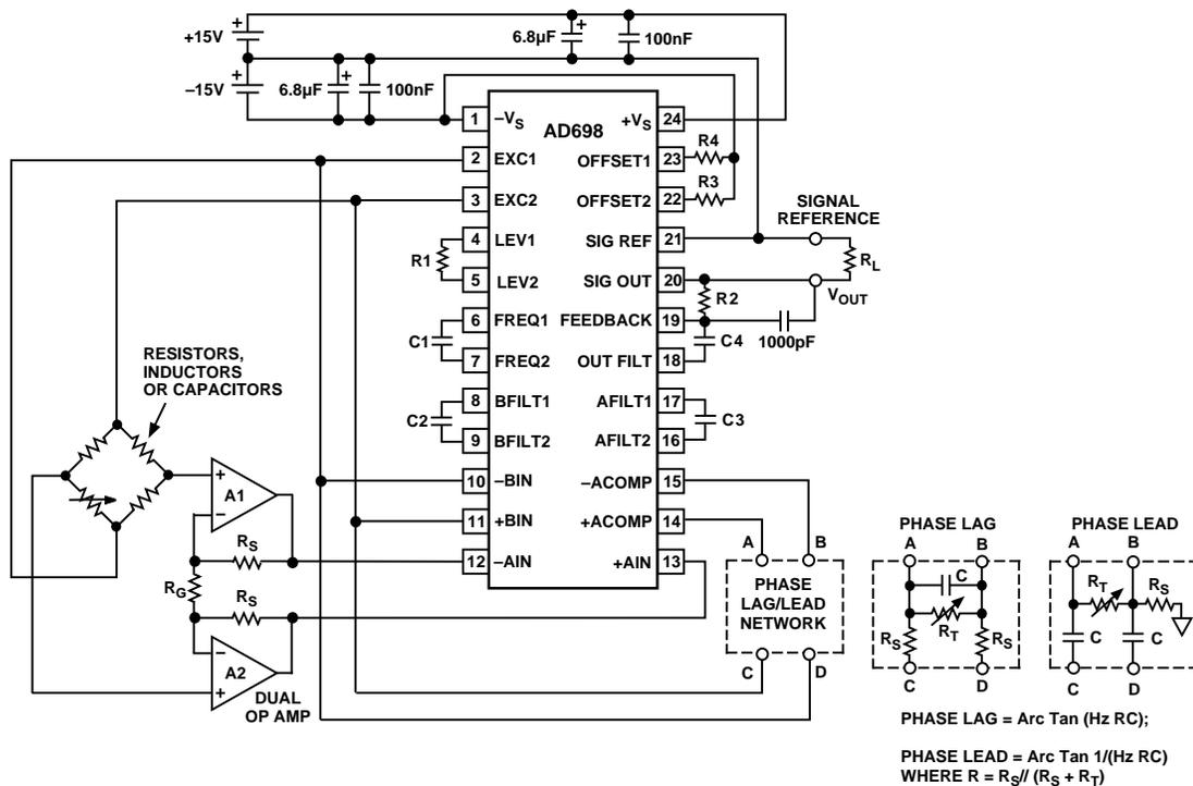
Figure 20. AD698 Interconnection Diagram for AC Bridge Applications
