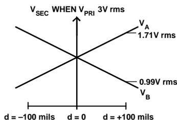
Figure 19. LVDT Secondary Voltage vs. Core Displacement
