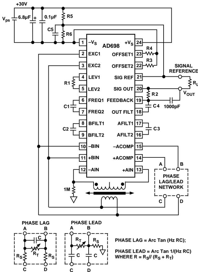
Figure 13. Interconnection Diagram for Single Supply Operation
