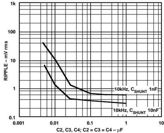
Figure 18. Output Voltage Ripple vs. Filter Capacitance
