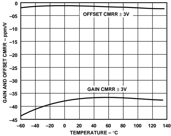
Figure 2. Gain and Offset CMRR vs. Temperature
