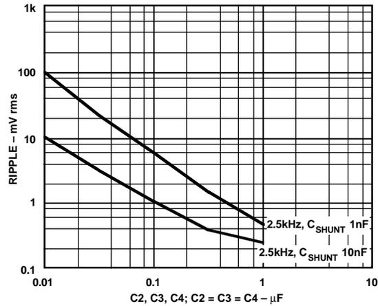
Figure 17. Output Voltage Ripple vs. Filter Capacitance
