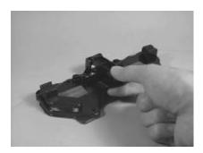
**8.** Press lever down to actuate splice. Remove the fiber from the foam holders first. Then remove the Fibrlok splice by pulling at the center of the splice
