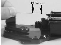
**3.** Use the cleaver to cut the fiber to a length of 12-13mm. Put the fiber into the fiber guide in the tool.
