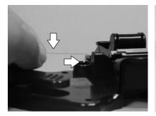
**4.** Insert the fiber into the splice until it stops.
