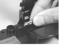
**2.** Put Fibrlok splice in the tool with the Fibrlok cap up. Strip 30–40mm of fiber buffer and clean the fiber with lint free wipe and alcohol.
