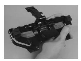
The Fibrlok splice can be installed without a work surface because the actuation tool can be held in one hand and actuated with the other.
