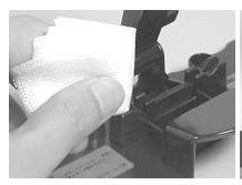
**1.** Clean both edges of the area where the splice is set in the tool with a lint free wipe and alcohol.
