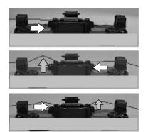
**7.** Hold down the arm where the second fiber will be inserted. Insert the second fiber until the first fiber bows as shown. Release the arm and push the first fiber to equalize the fiber bows as shown.
