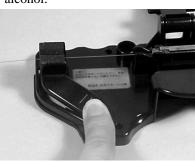
**5.** Press arm down and place fiber into open foam holder. Release arm so that the foam holder retains the fiber.
