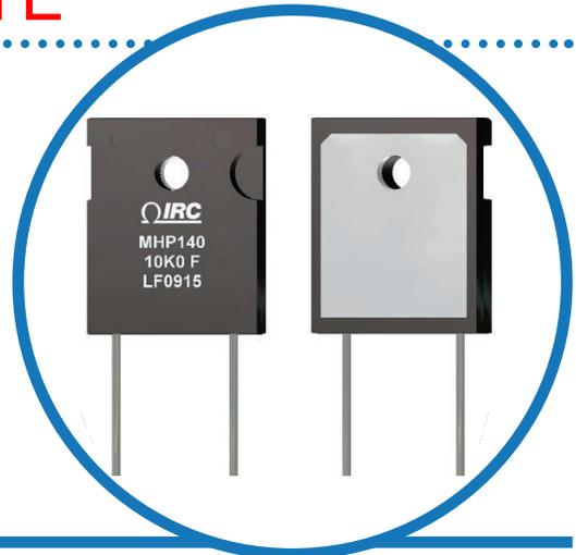
IRC's MHP series resistors satisfy demanding applications for accurate and stable power resistors housed in the convenient TO-247 case. The resistance element is isolated from the mounting tab by an alumina ceramic layer, providing very low thermal resistance and ensuring high insulation resistance between terminals and metal back plate. The non-inductive design makes these products especially useful in high frequency and high speed pulse applications.
