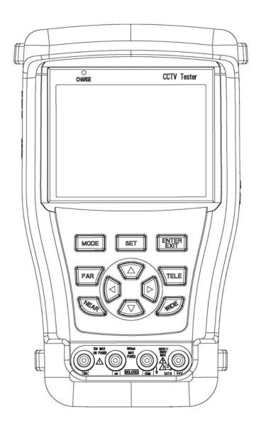
3.5" TFT LCD Colour Monitor with LED Back light, Composite Video In/Out BNC, 12volts output for Camera, Colour Pattern Generator, Multi-meter, PTZ controller, LAN cable tester, Audio input for Microphone checking. Carry bag, Straps, Rechargeable Li-Polymer Battery, Test leads.
