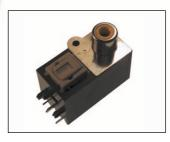
OTJ-6/ORJ-6 Dual SPDIF RCA and Optical Transmitter and Receiver Jack. Right angle PCB mount with self tapping hole for panel mounting. Hinged shutter. Several different colored inserts available.
