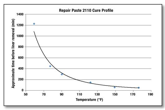
Approximate minimum time required as a function of temperature before the 3M Repair Paste Release Liner can be removed from curing Repair Paste 2110.
