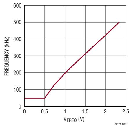
Figure 7. Relationship Between Oscillator Frequency and Voltage at the FREQ Pin
