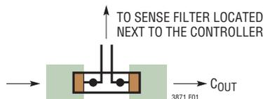
Figure 1. Sense Lines Placement with Sense Resistor
