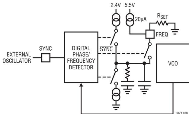
Figure 8. Phase-Locked Loop Block Diagram
