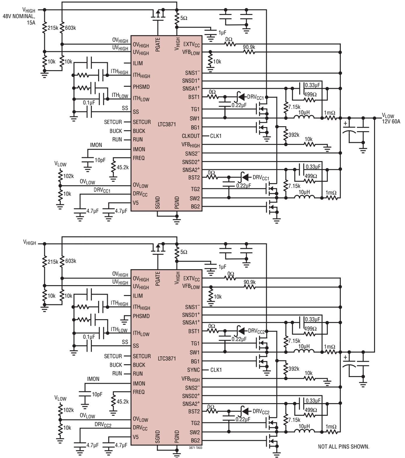
Figure 12. High Efficiency 12V, 60A 4-Phase Supply
