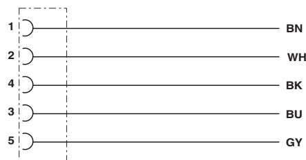
Contact assignment of the M12 socket
