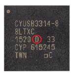
Cypress maintains traceability of product to wafer level, including wafer fabrication location, through the lot number marked on the package.
