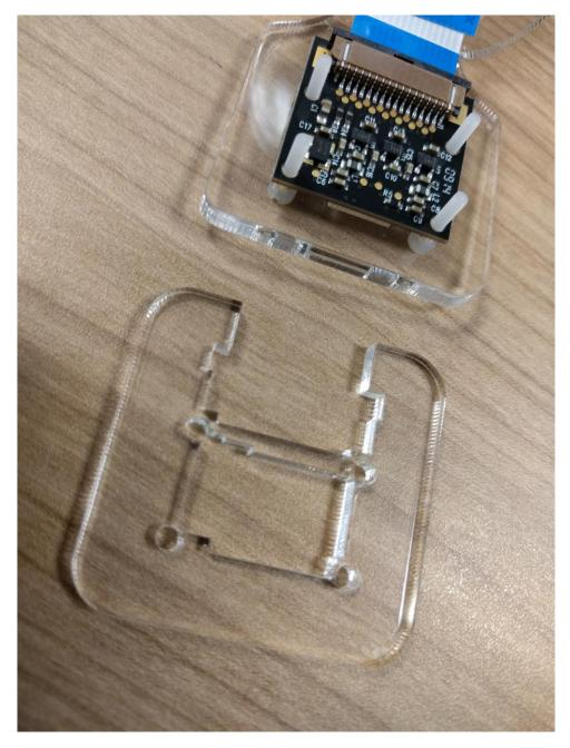
5. Place the Perspex back plate over the 4 nylon screws such that the open slot in the Perspex back plate is over the camera ribbon cable.
