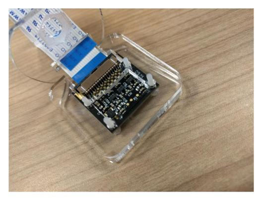
6. Take 4 nylon nuts, and use them to secure the Perspex back plate in place. The remaining 8 nylon nuts are not required.
