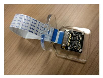
4. Take the Perspex back plate, and orient it such that the cut outs in the central rectangular hole are aligned as shown in the image below. Because of the placement of chips on the rear of the camera board, this Perspex back plate will only fit correctly if fitted the right way round.
