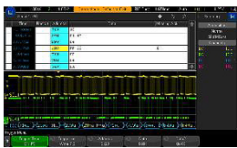
Figure 15: I 2 C decode and trigger
