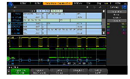
Figure 19: Multi-bus time aligned decode
