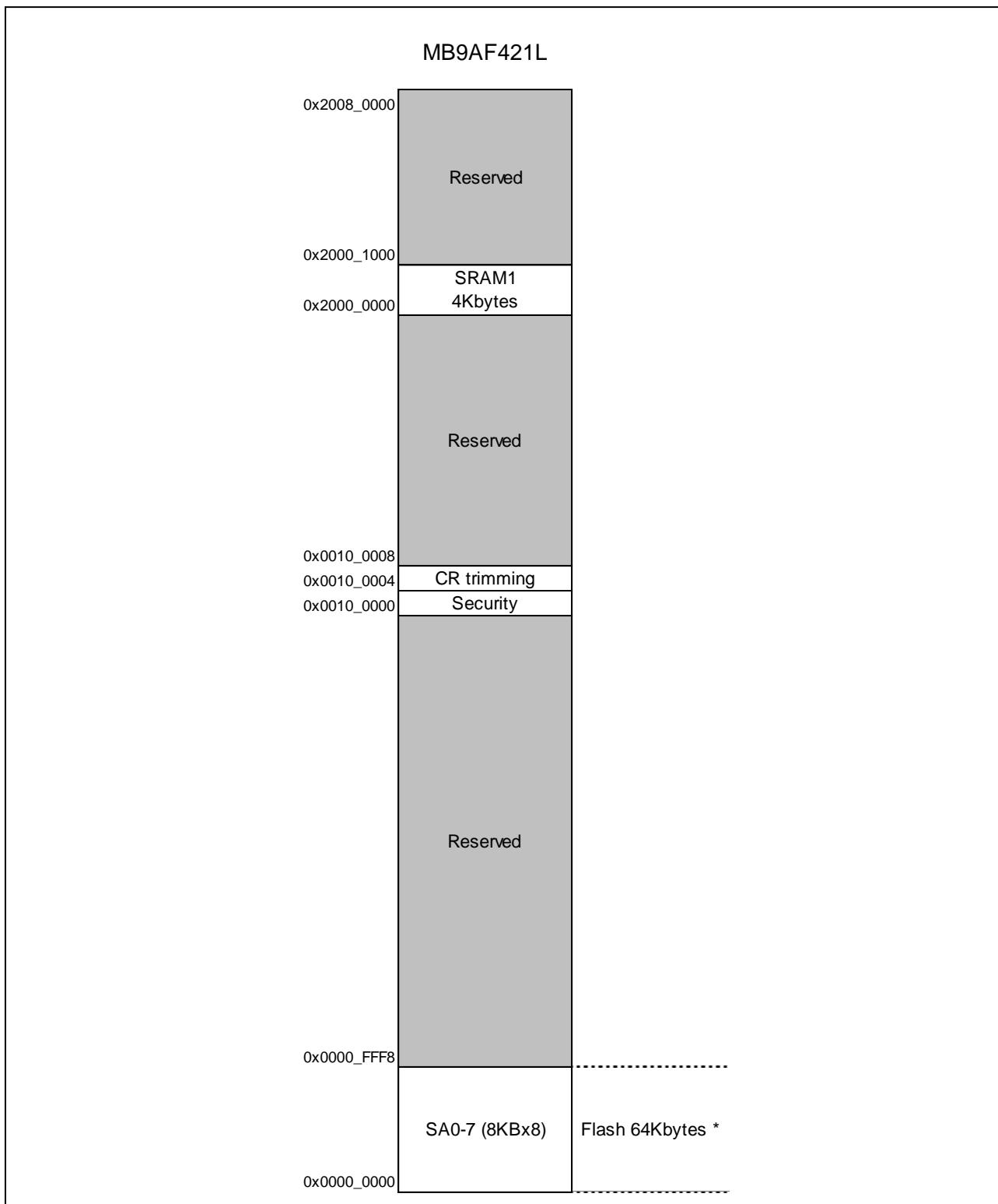
\*: See MB9A420L/120L/MB9B120J Series Flash Programming Manual to confirm the detail of Flash memory.
