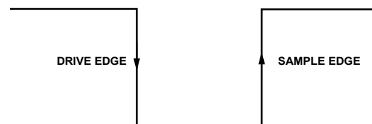
Figure 45. SPI Mode 3 SCLK Edges
