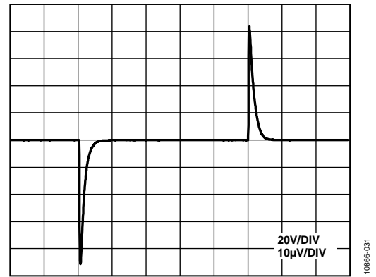
Figure 31. Operational Amplifier Load Transient Response (100 µA Load Change)
