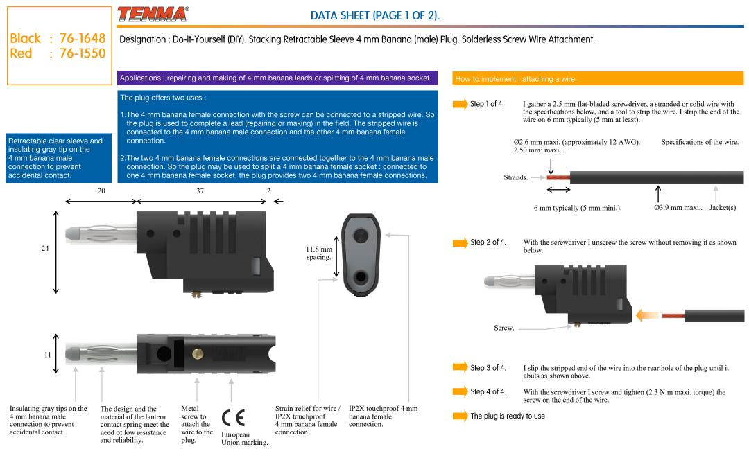
The 4 mm banana male connection complies with the 4 mm banana sockets of the worldwide most famous manufacturers. The 4 mm banana female connections comply with the 4 mm banana plugs of the worldwide most famous manufacturers.
