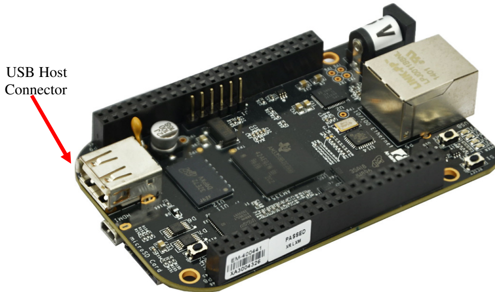
Figure 53 USB Host Connector
