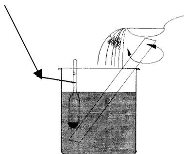
Put in a densimeter and pour in 1 soupspoon of anhydrous sodium hydroxide. Stir with the plastic stirrer (which can be a plastic off-cut).
