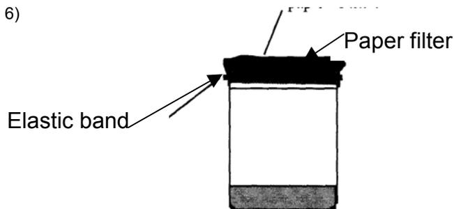
Position and attach filter paper on the container so that the sludge remains in the container when it is turned upside down.
