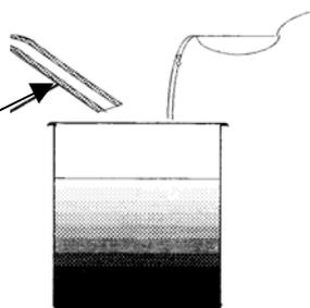
Use the pH paper\* to accurately check that the mixture is neutral. Add small quantities of sodium hydroxide whilst monitoring the change in colour of the pH paper. When the pH stabilises at around 7 after mixing, we can observe that a brown sludge is deposited at the bottom of the bucket, whilst the liquid becomes increasingly clear.
