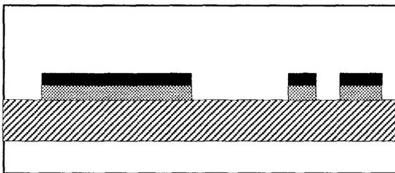
The iron perchloride has attacked all parts of the copper, which were not protected.
