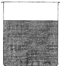
Pour 2 litres of waste iron perchloride into the 2.5 litres plastic bucket. Place all of this in a sink for maximum safety.
