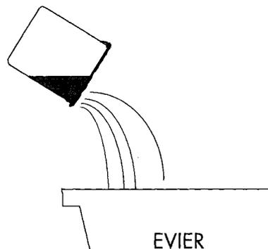
Pour out the clear liquid into the sink (it is salt water and can be poured to waste). Put the sludge in a plastic container. This sludge can be thrown away either in a landfill or spread on a field. In town, it may be disposed of using normal waste disposal procedures.
