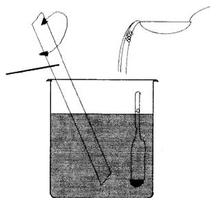
Wait for 2 minutes then add the sodium hydroxide little by little whilst stirring until the densimeter shows a pH approximately equal to 7 (the "zero" graduation of the densimeter arrives at the liquid surface). Again wait for a few minutes.
