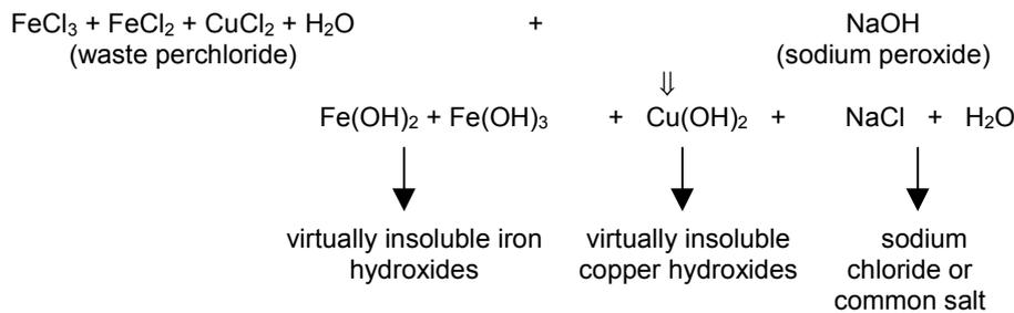
When the mixture is carried out correctly in the right proportions, in other words for the pH to be neither acidic nor basic, we should note that :
