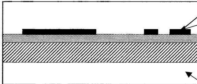
The opaque film is obtained either using an adhesive tape or using a photosensitive layer, which has been exposed to light and then developed.
