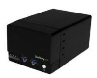
The S352BU33HR 2-Bay RAID Enclosure lets you build an external RAID array using two 3.5" SATA hard drives, and add it to your computer through USB 3.0.
