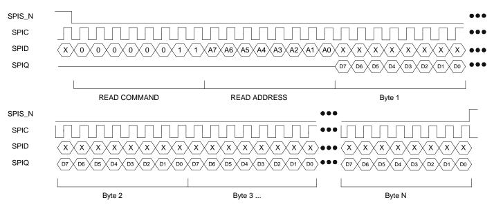
Figure 18. SPI Multiple Read
