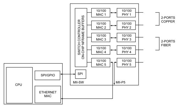
Figure 4. Using KSZ8895FQX for Dual Media Converter
