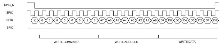
Figure 15. SPI Write Data Cycle
