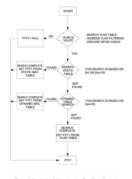
Figure 10. Destination Address Lookup Flow Chart, Stage 1
