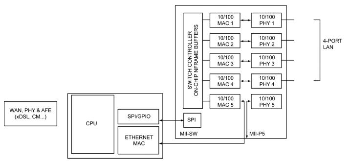
Figure 2. Integrated Broadband Router
