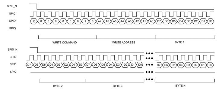
Figure 17. SPI Multiple Write
