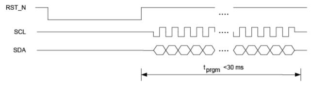
Figure 14. KSZ8895MQX/RQX/FQX/ML EEPROM Configuration Timing Diagram
