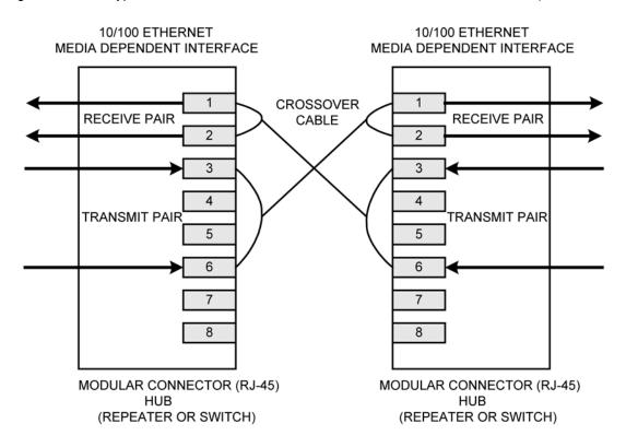
Figure 6. Typical Crossover Cable Connection
