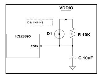
Figure 34. Recommended Reset Circuit
