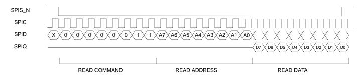
Figure 16. SPI Read Data Cycle
