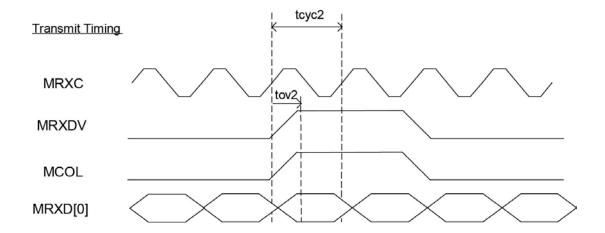
Figure 22. SNI Output Timing
