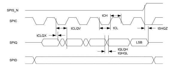
Figure 30. SPI Output Timing
