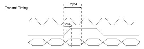
Figure 26. PHY Mode MII Timing – Data Transmitted from MII
