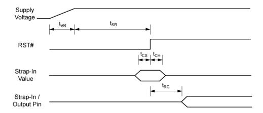
Figure 33. Reset Timing
