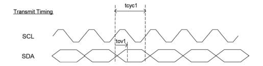
Figure 20. EEPROM Interface Output Transmit Timing Diagram
