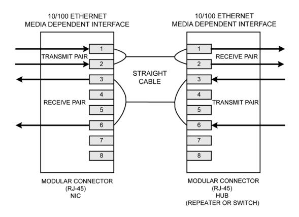
Figure 5. Typical Straight Cable Connection
