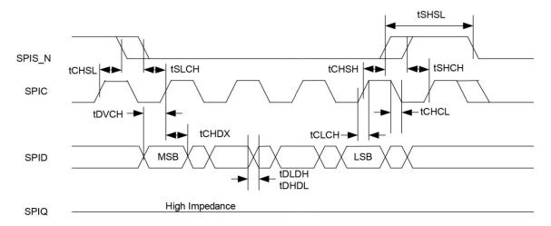
Figure 29. SPI Input Timing
