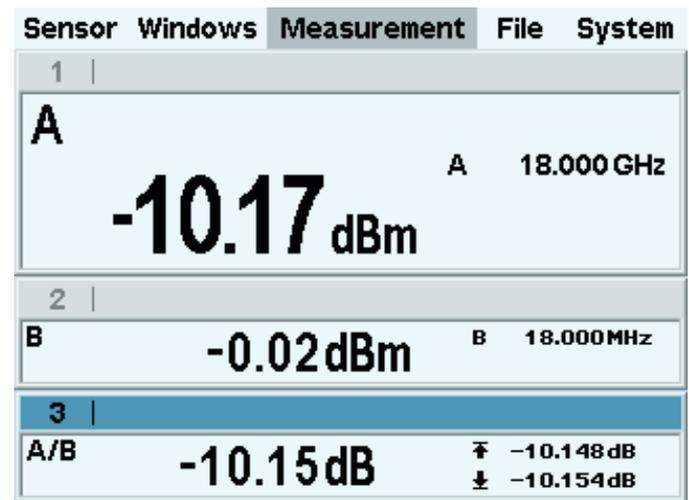
Determination of the power of an EDGE burst with the R&S®NRP-Z81 wideband power sensor using the gate function; exclusion of the training sequence in the center of the signal.
