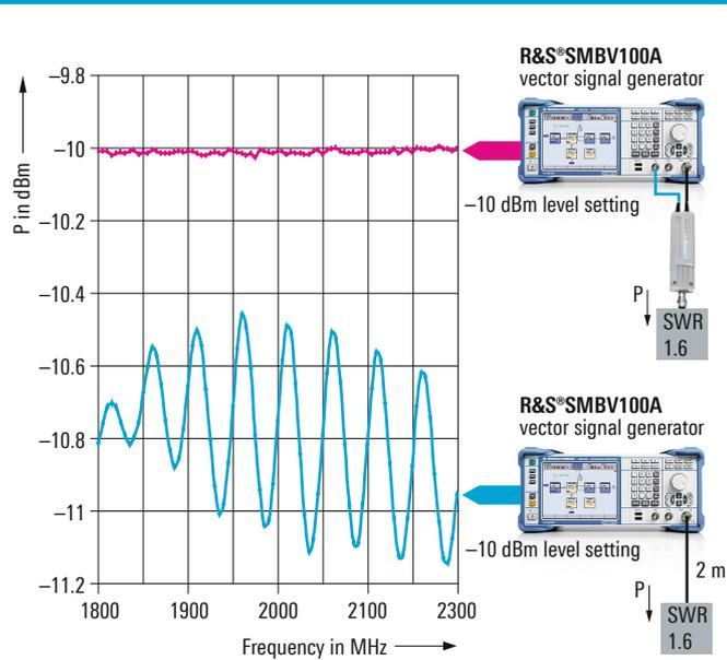
Upper graph: using the R&S®NRP-Z28, with activated user correction;
