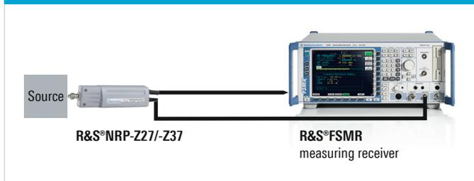
R&S®FSMR measuring receiver with R&S®NRP-Z27 power sensor module.
