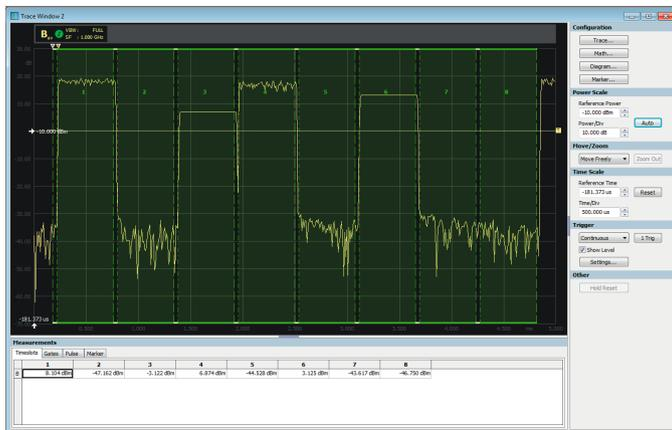
Statistical analysis of an LTE signal using the R&S®NRPV.
