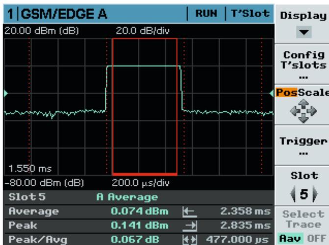
Numerical display of two continuous average measurements and their relation.
