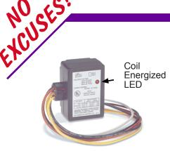
The **SSU-RIC-1** Relay, SPDT, provides 10.0 Amp resistive form C contacts. The relay coil may be energized by one of three input voltages: 24VDC, 24VAC, or 115VAC. **SAE PN# SSU-RIC-1**
