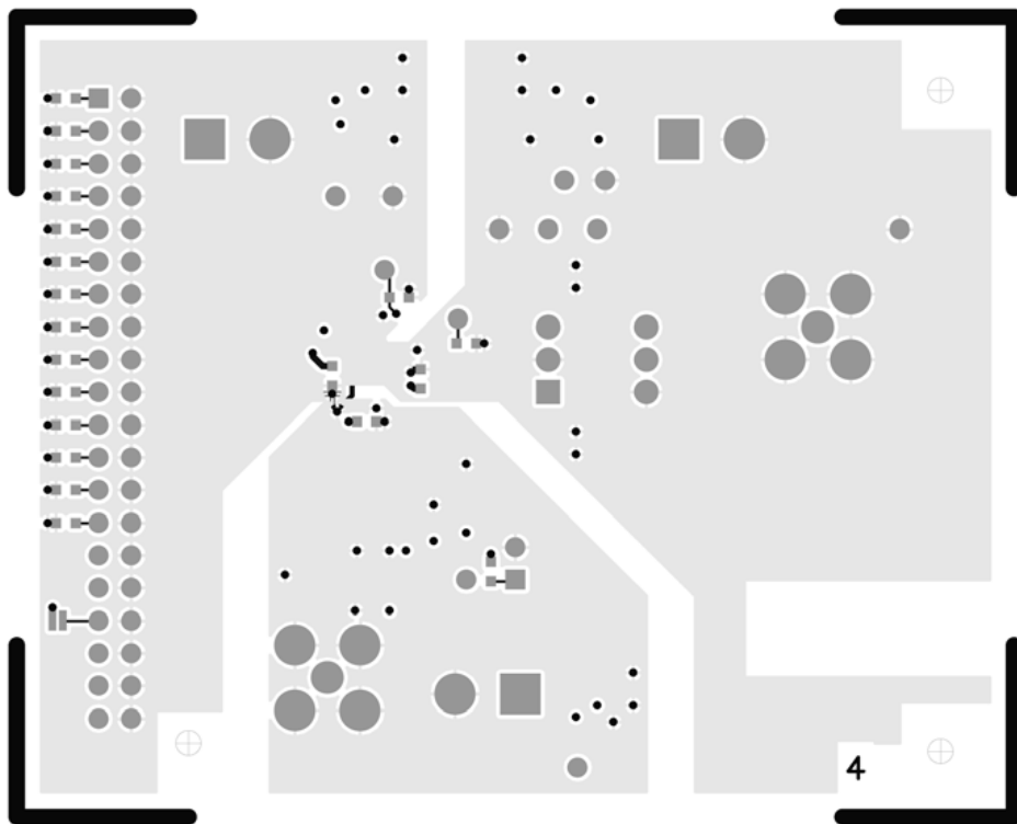
Figure 36. Evaluation Board Layout—Secondary Side
