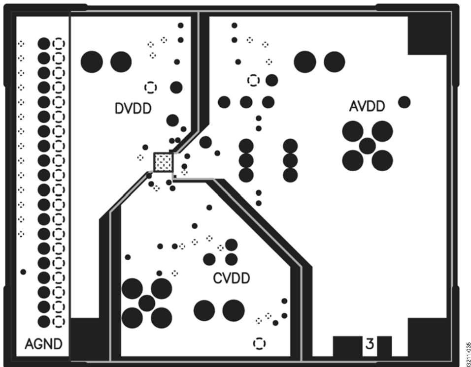
Figure 38. Evaluation Board Layout—Power Plane
