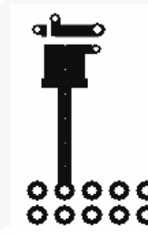
Figure 5. Minimum Pads of 2-ounce Copper
