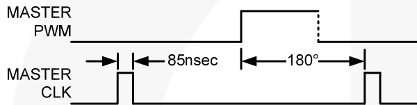
Figure 35. Synchronization Timing Diagram
