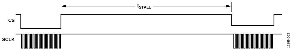
Figure 3. Stall Time and Data Rate
