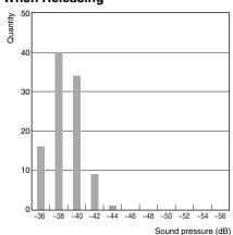
Sample: G5RL-1A-LN 12 VDC Number of relays: 100 pcs Range:A weighted sound pressure level, Fast, Max. hold Device connected to coil: Diode Testing environment:Room temperature and
