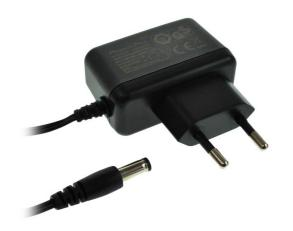
This switch mode power supply is rated to 6W maximum, providing a regulated 9vdc output at up to 0.66A with no minimum load. The unit meets latest CoC Tier 1 / Level VI efficiency standards and will be uprated to CoC Tier 2 requirements before the requirement is made mandatory.
